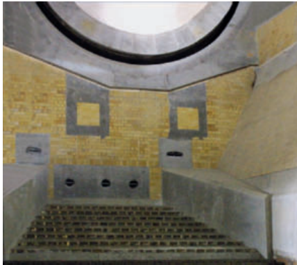
3 Static cooler grate
