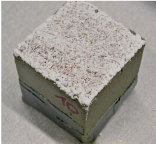
3 Crystallization of sodium chloride salt on brick in the absence (left) and in the presence (right) of crystallization inhibitor in the salt solution
