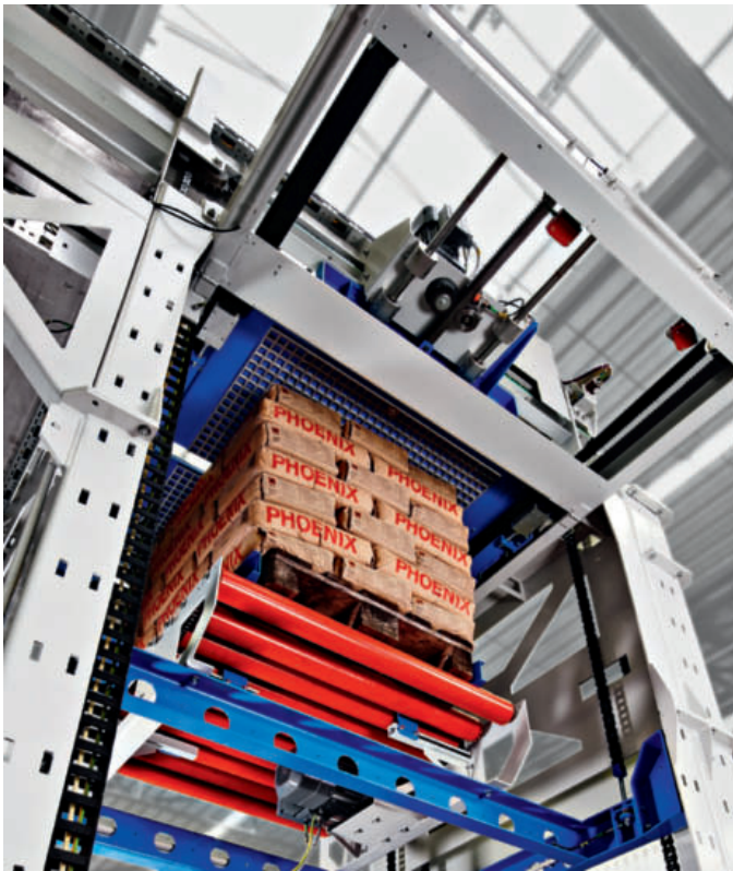
4 The Beumer paletpac forms exact, stable and thus space-saving bag stacks
