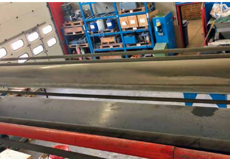
5 Claudius Peters Fluidcon system for pneumatic conveying
