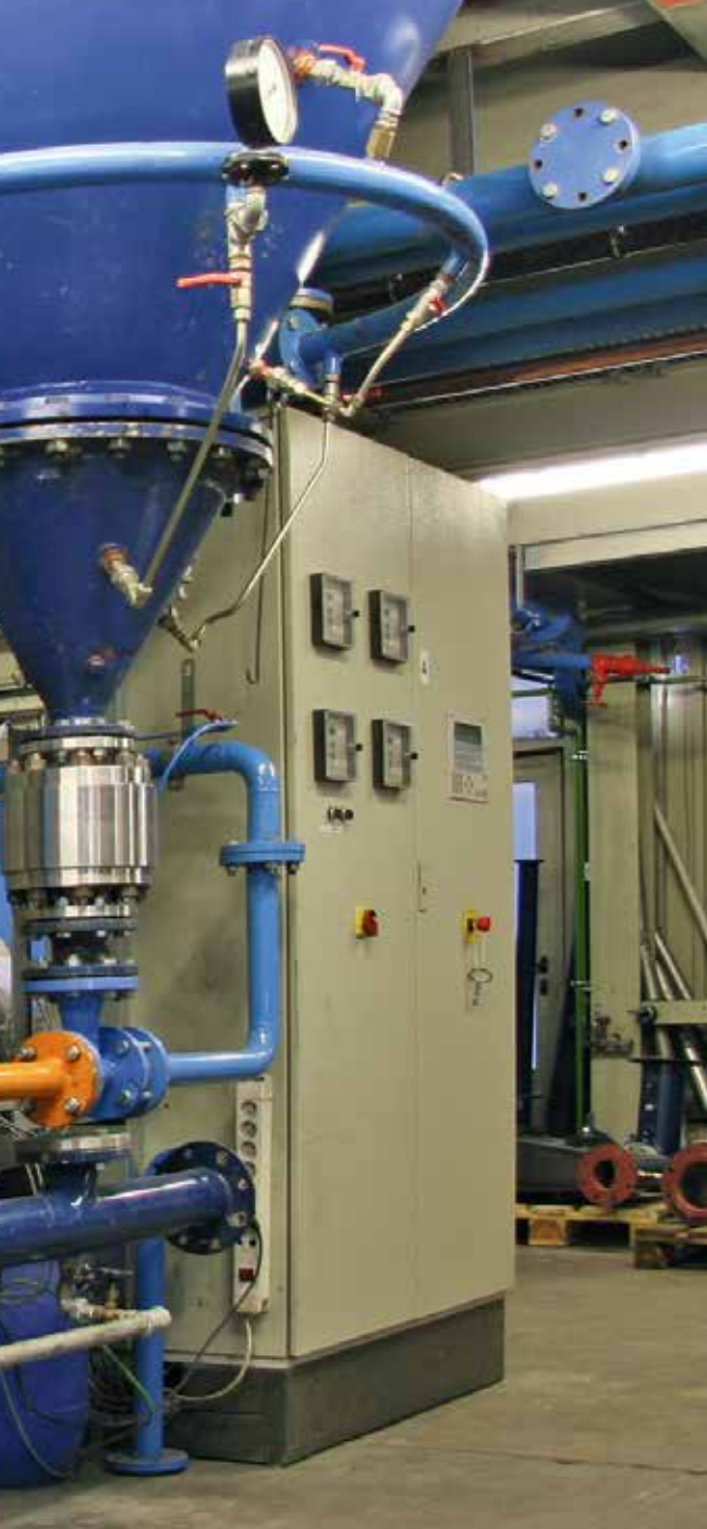
Test stand in the Claudius Peters technical center for pneumatic conveying
