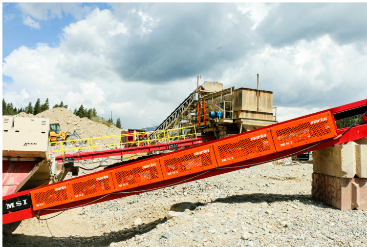
7 Conveyor guarding prevents reach-in, but also constrains fugitive debris to under the system
