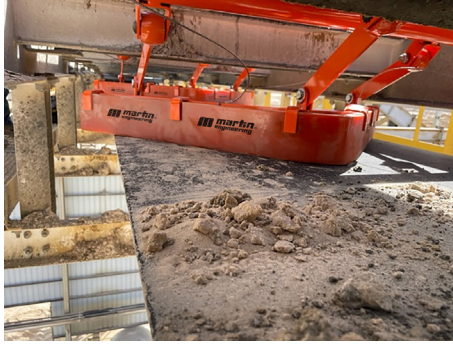
6 The workhorse of tail pulley protection, the V-plow safely clears debris without harming the belt
