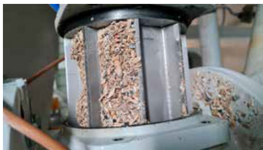
5 Bad particle shapes, coarser granulometry and high impurities content
