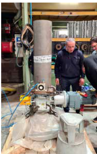
9 Workshop test of rotary valves
