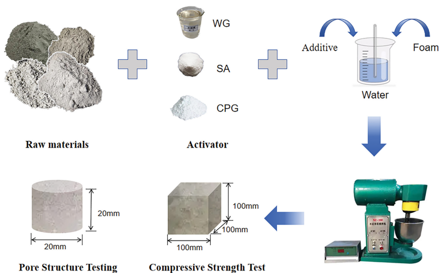
Figure 4 Preparation process of phosphogypsum foam concrete specimens
