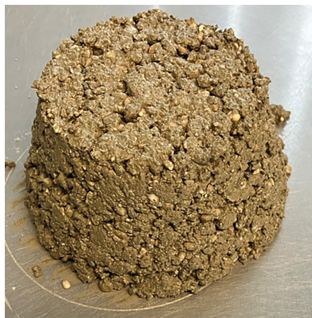
Figure 2 (a) w/c = 0.6 . The mortar is still compact and has a light, shiny water film. (b) w/c = 0.55 . The mortar cake falls apart slightly and looks very dry and brittle
