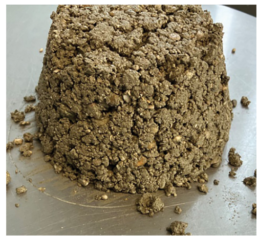
Figure 2 (a) w/c = 0.6 . The mortar is still compact and has a light, shiny water film. (b) w/c = 0.55 . The mortar cake falls apart slightly and looks very dry and brittle
