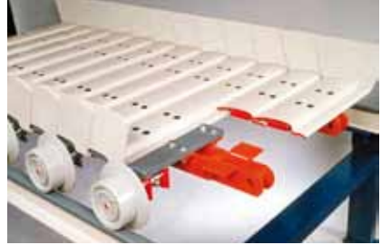
12 Aumund plate feeder type BPB
