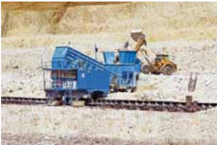
9 Samson material feeder – the mobile feed point to field conveyor
