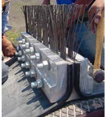
2 Automated belt punch at Aumund works, Rheinberg/Germany, and Aumund clamping device on site
