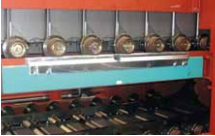
15 Weigh rail load cell mounted and Aumund weigh feeders at TXI Oro Grande
