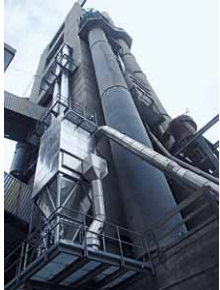
6 Cooling duct and bag filter for sorbent separation
