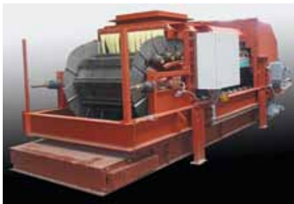
20 Aumund weigh feeder with spillage returns
