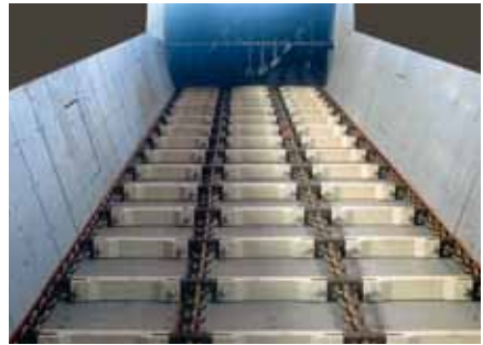
18 Underground hopper with Aumund PKF feeder and armoured chain feeder type PKF
