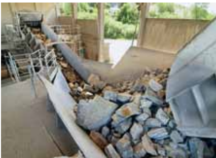
6 Aumund heavy duty feeder type BPB-SF
