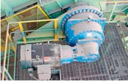
8 Planetary and helical reduction gear (photo Aumund)
