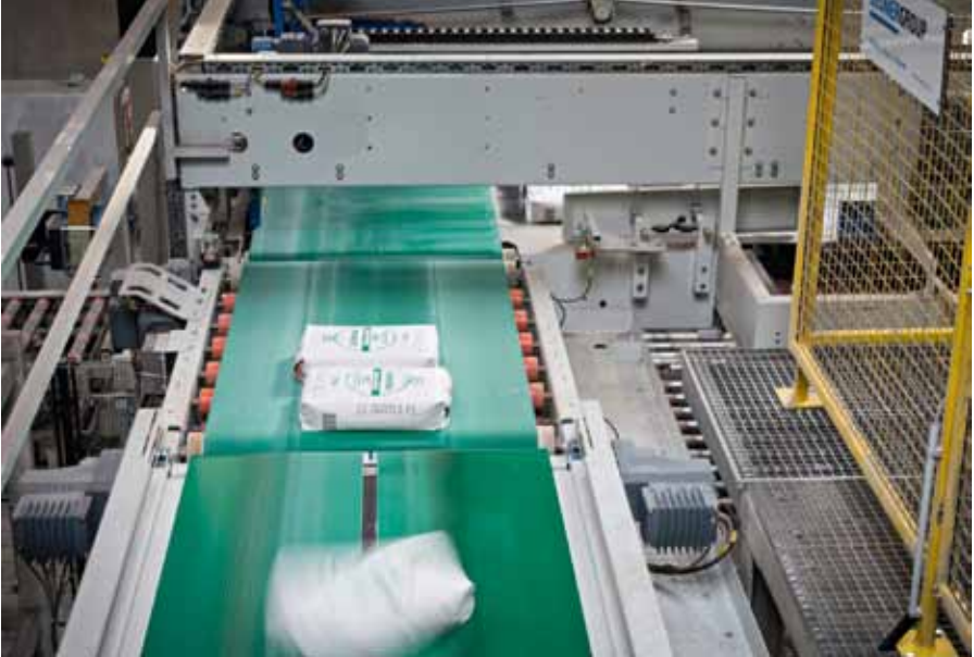
2 The twin-belt turning device: Two parallel belt conveyors, driven with different speeds during the turning process, bring the bags gently into the required position
