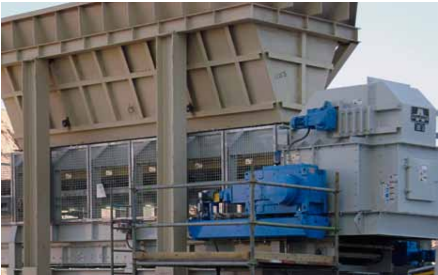
16 Aumund BPB-S plate feeder for shovel loading
