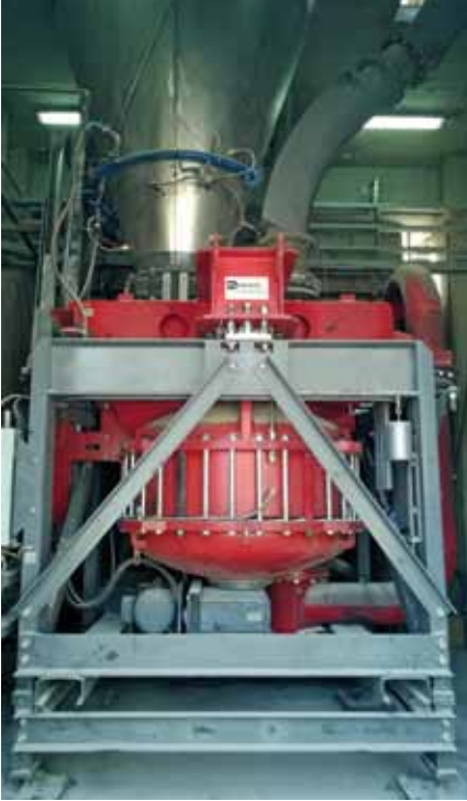
3 Perfect dosing with rotor weighfeeder Pfister DRW
