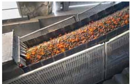
3 Aumund pan conveyor type KZB for handling of hot material
