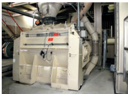
1 A dry powder batch mixer of type DMX 3600 has proven itself for years in a German dry mortar plant
