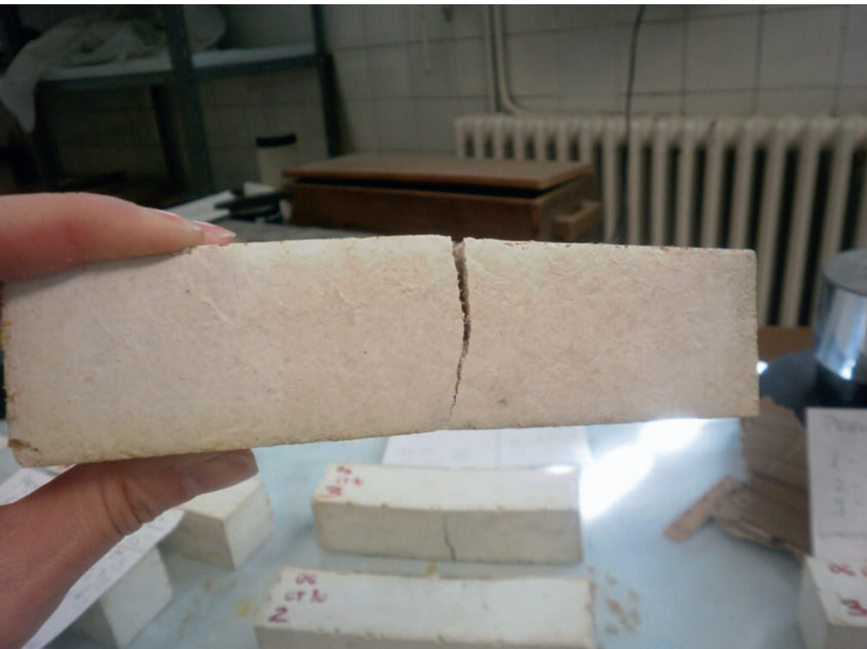
9 CT sample fracture due to flexural strength
