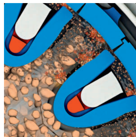
3 Functional principle of the rotor impact mill of type RPM
