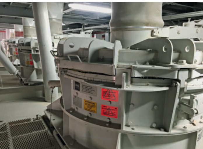
1 Five BHS rotor impact mills of type RPM 1513 are operating at Siam Mortar's Khaeng Khoi III, Saraburi plant
